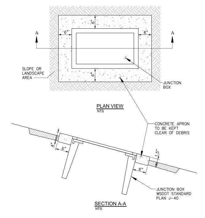
FOR NEW CONSTRUCTION AND MODIFICATION OF EXISTING J-BOX
