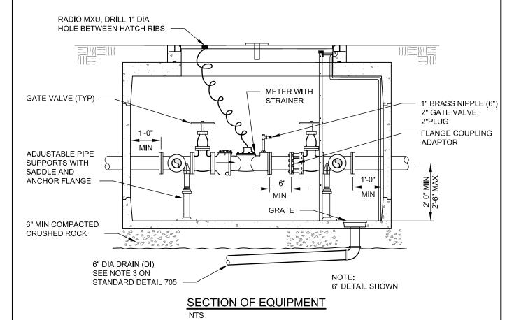
SET COVER SLAB FLUSH WITH SIDEWALK OR CURB ELEVATION IF LOCATED IN LAWN AREA. SET COVER SLAB APPROXIMATELY 2" ABOVE FINISHED GRADE IF LOCATED IN LANDSCAPING AREA.
