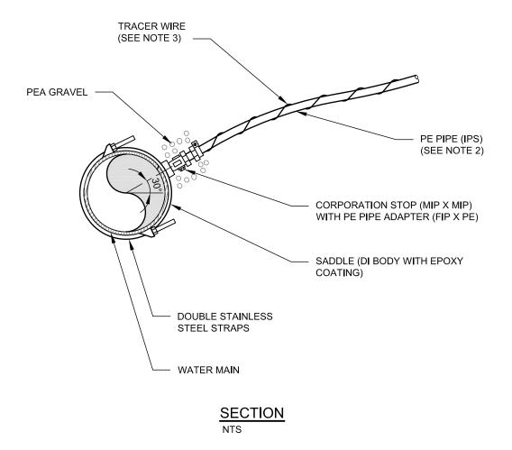
IPS = IRON PIPE SIZE FIP = FEMALE IRON PIPE THREAD MIP = MALE IRON PIPE THREAD
