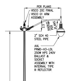
PAINT SPECIFICATIONS: ALL CAST IRON AND STEEL LIGHT POLE PARTS ARE TO BE FACTORY PRIME PAINTED WITH "TNEMEC" PRIMER AND FACTORY FINISH PAINTED WITH "TNEMEC" PEKING BLUE, ENDURASHIELD #F175B2705A 8556A, OR APPROVED EQUAL.
