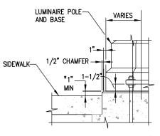
\* TOP OF FOUNDATION TO BE LEVEL, 1" MIN HEIGHT ABOVE TOP OF SIDEWALK
