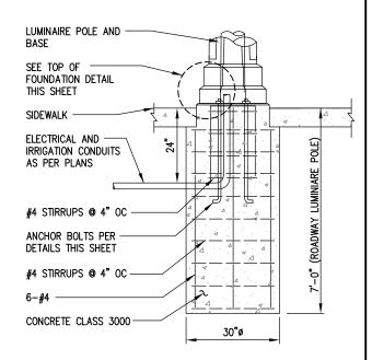
LUMINARE POLE AND FOUNDATION DETAIL NTS
